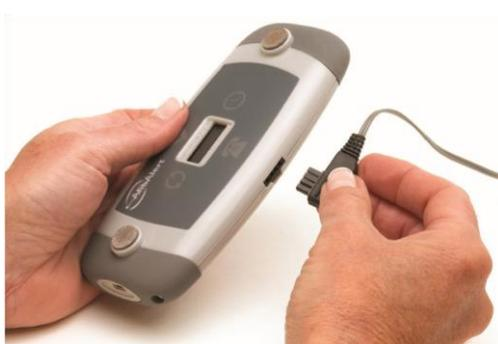
3.3 The cable can only be inserted in one direction.
