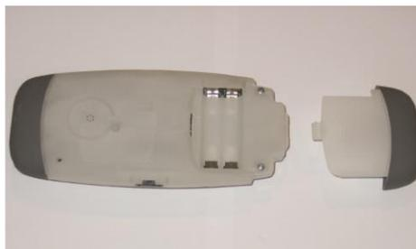
6.1 The battery cover slides off by applying a slight pressure on the arrow.
