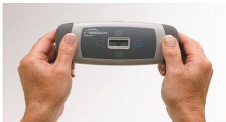
3.2 Press thumbs firmly on the electrodes. The Blue light will illuminate during the test.
