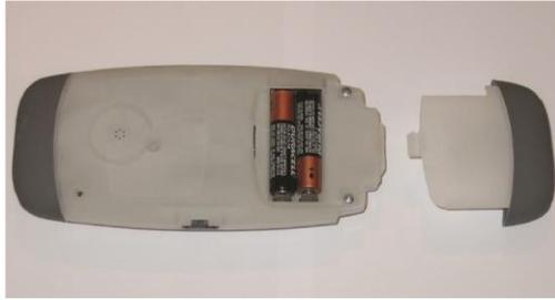
6.2 Insert 2 'AAA' Alkaline batteries in either direction.
